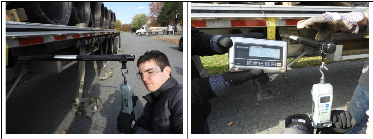
Figure 7. Example of the procedure used to evaluate the force exerted on the lever when three levels of strap tension are reached
