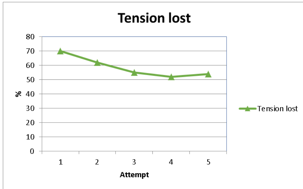
Figure 16. Representation of the percentage of tension lost during the initial tightening of the strap for each attempt with the TRADITIONAL winch. Refer to Figure 15
