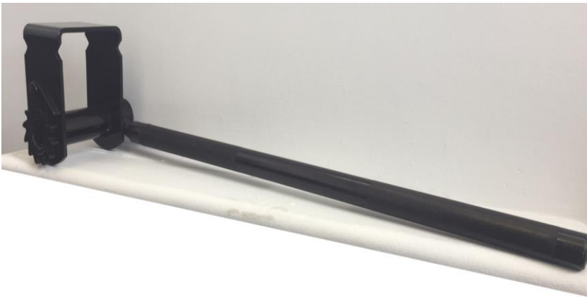
Figure 1. TRADITIONAL winch system with winch bar
